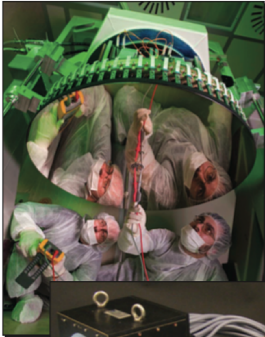
Lab testing of the Large Binocular Telescope's adaptive secondary mirror system with 672 actuators
