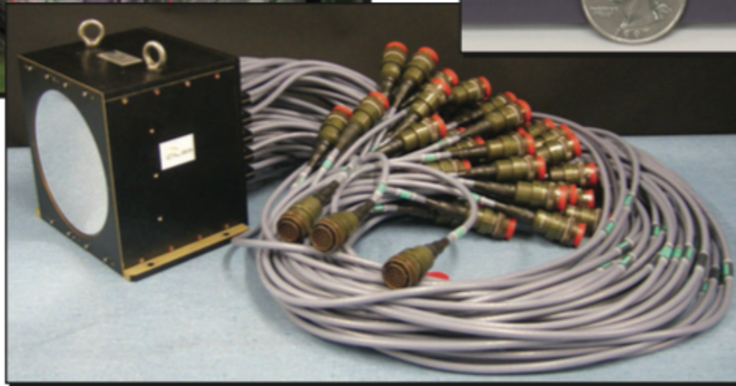
Piezo high-order 1,377-actuator DM for SPHERE
