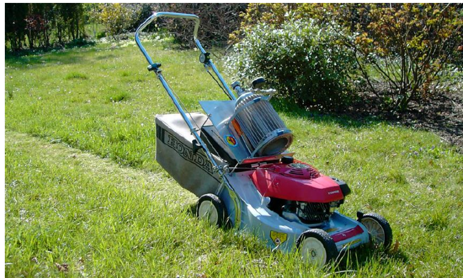
Hydrogen powered lawn mower (K. Yvon).
